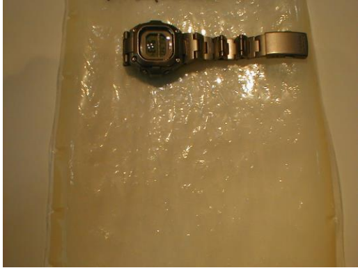
Figure 7: A three-layer sheet sample with poor layer distribution and distortion
